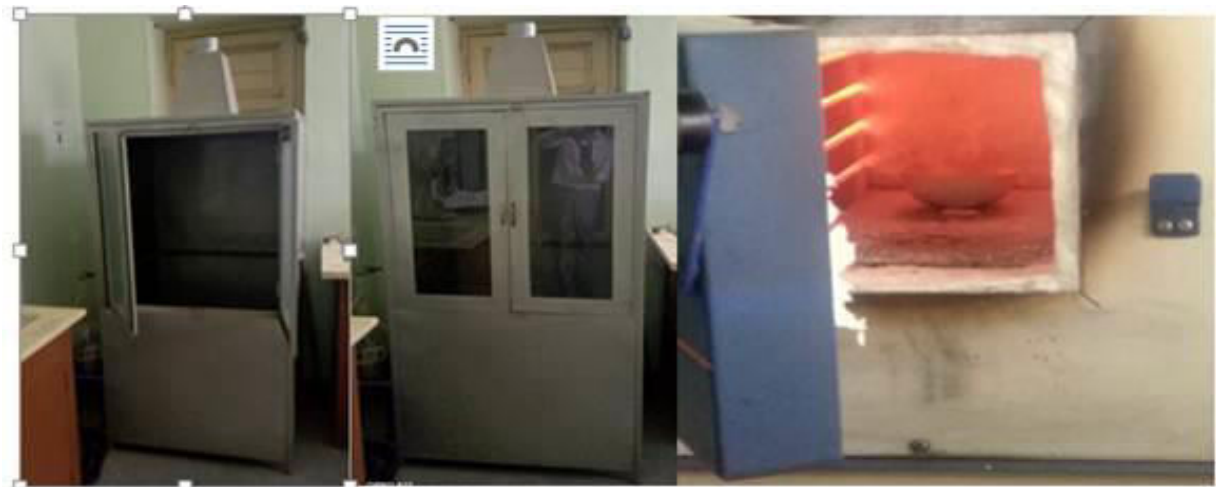
Figure 4. Fabricated chamber & furnace used for combustion synthesis.
