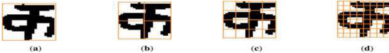
Fig. 2 : A character image : a) one zone b) 4 zones c) 16 zones and d) 64 zones.
